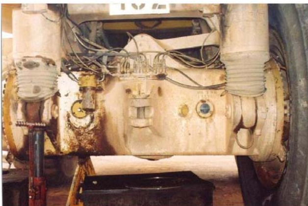
Haul Truck Rear Differential
