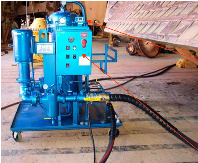
40 GPM Filtration System
