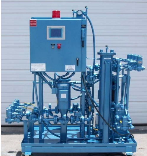
8 GPM Fuel Polishing System
